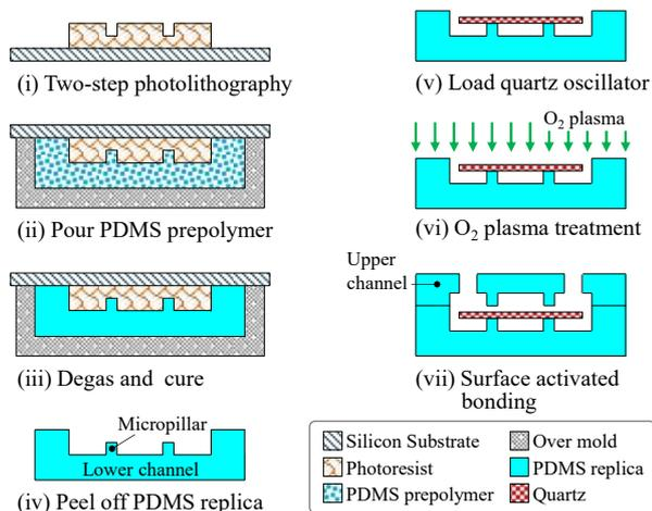
Fig. 2 Fabrication steps using the photoresist mold.
