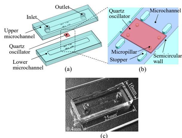
Fig. 1 (a) Exploded view of the PDMS RAMNE-Q biosensor chip, (b) Enlarged view, (c) Assembled chip.
