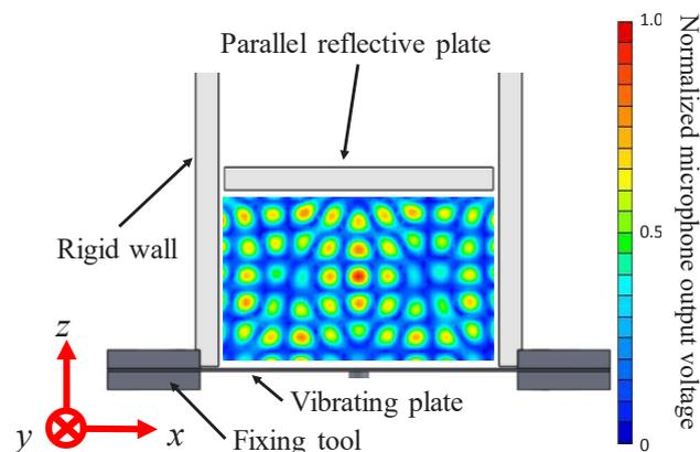
Fig. 4. Sound pressure distribution in the  $x$ - $z$  plane with a parallel reflective plate.
