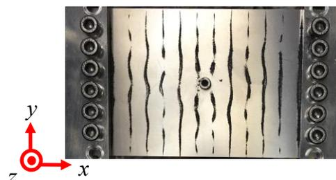
Fig. 3. Chladni figure of a vibrating plate with two fixing tools ( $N_W=9$ ).
