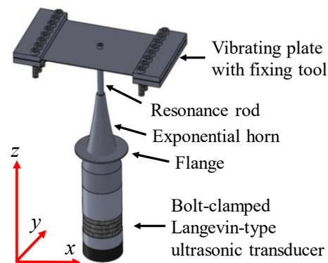
Fig. 1. Schematic of the ultrasonic source.
