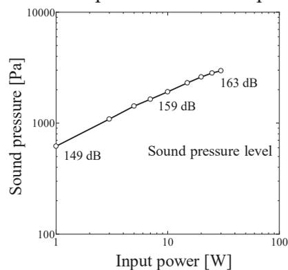
Fig. 5. Relationship between input power and sound pressure.
