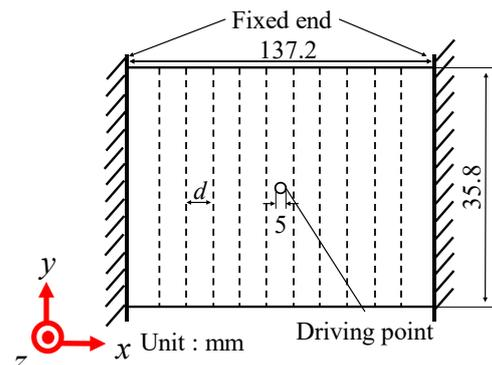
Fig. 2. Schematic of the vibrating plate ( $N_W=9$ ).
