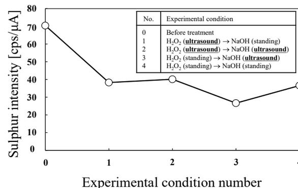
**Fig. 4.** Sulphur intensity of bitumen after treated with H<sub>2</sub>O<sub>2</sub> (30 wt. %) and NaOH with/without ultrasound irradiation
