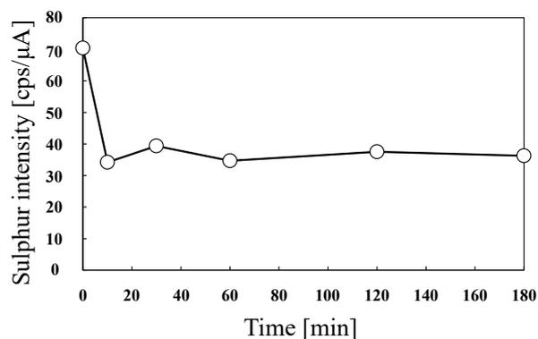
**Fig. 2.** Change of sulphur intensity by NaOH reaction time. (H<sub>2</sub>O<sub>2</sub> reaction time: 10 min)
