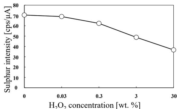
**Fig. 3.** The effect of H<sub>2</sub>O<sub>2</sub> concentration on the desulphurization of bitumen
